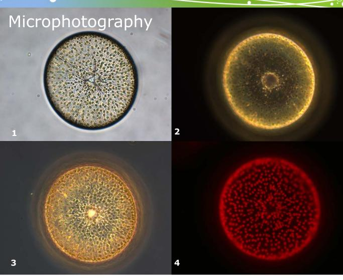
**1: Brightfield Microscopy:** Simplest microscopy illumination technique. Specimen is illuminated from below and observed from above. Specimens typically appear as dark shapes against a bright background.
